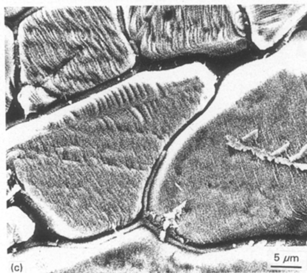
Figure 7 Scanning electron micrographs of polished and thermally etched surfaces of doped samples sintered at (a) 1325 °C, (b) 1350 °C and (c) 1400 °C.
